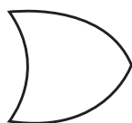
The standard symbol of the OR Gate
